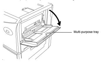
2. Open the sub tray and adjust the paper guides according to the width of the paper to be fed.
